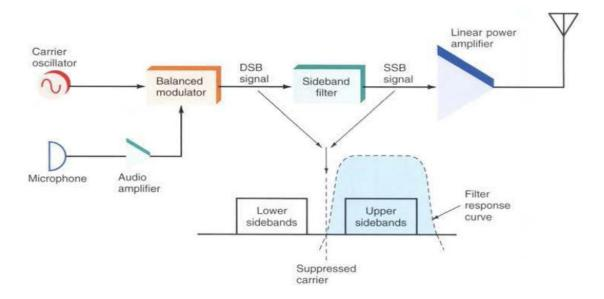
(b) An SSB signal is generated by modulating a 5-MHz carrier with a 400-Hz sine tone. At the receiver, the center frequency of the filter needed to pass the lower sideband is? (3 marks)
